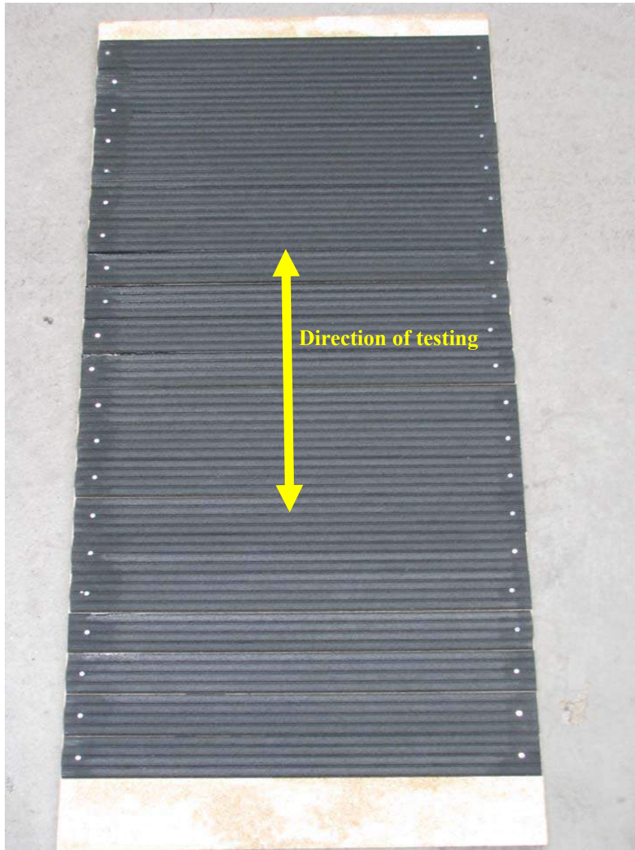
Figure 1: General view of Ecoglo N1070 slip resistant strips fastened to particle board for testing. Arrow indicates direction of testing..
