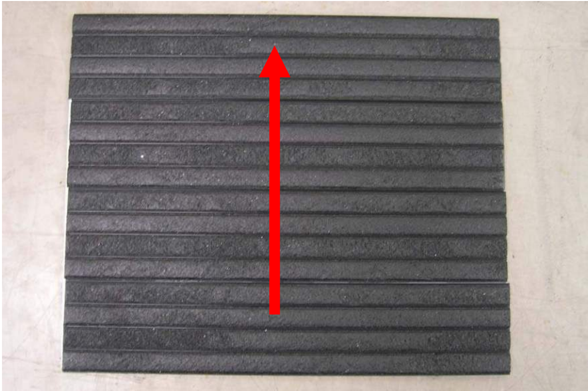
Figure 1: General view of Ecoglo N1070 product. Arrows indicate direction of wet testing.
