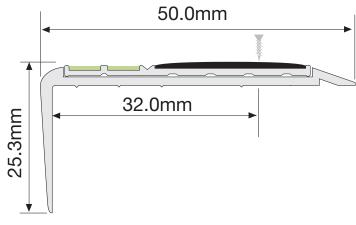
The F9-175 Step Nosing is designed to ensure visibility of steps in escape routes for compliance with International Fire Code (IFC) and any performance based building codes. The Step Nosing will be effective in all light conditions including during failure of the main lighting.
