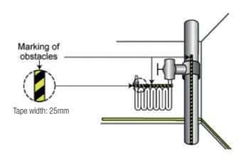
The UL-HZ2503 Hazard Tape is designed to ensure visibility of obstacles in escape routes for compliance with NFPA 101 Life Safety Code (NFPA 101) and International Fire Code (IFC). The Hazard Tape will be effective in all light conditions including failure of the main lighting.
