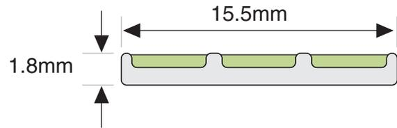
The G3-001 Guidance Strip is designed to ensure visibility of specified building features in escape routes for compliance with NFPA 101 Life Safety Code (NFPA 101) and International Fire Code (IFC), and any performance based building codes. The Guidance Strip will be effective in all light conditions including during failure of the main lighting.
