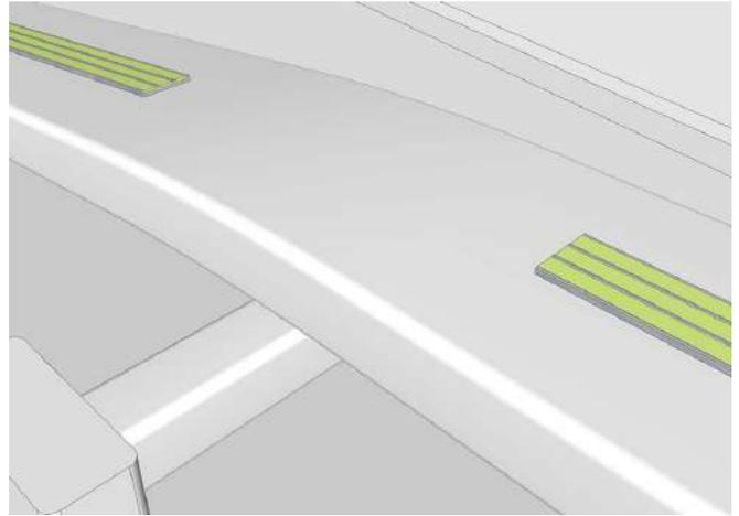
Do not bend guidance strips over bends. Set the strip 50mm from the bend.
