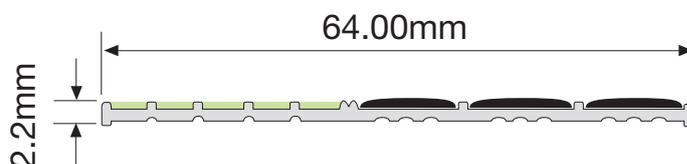
The E15-073 Step Edge Contrast is designed to ensure visibility of steps in escape routes for compliance with NFPA 101 Life Safety Code (NFPA 101) and International Fire Code (IFC). The Step Edge Contrast will be effective in all light conditions including during failure of the main lighting.
