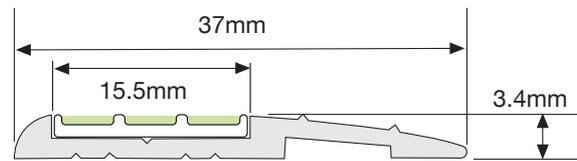
The T6-101 Path Marker is designed to ensure visibility of specified building features in escape routes for compliance with NFPA 101 Life Safety Code (NFPA 101) and International Fire Code (IFC), and any performance based building codes. The Path Marker will be effective in all light conditions including during failure of the main lighting.
