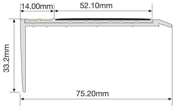
**The F15-175 Step Nosing is designed to ensure visibility of steps in escape routes for compliance with International Fire Code (IFC), and any performance based building codes. The Step Nosing will be effective in all light conditions including during failure of the main lighting.**
