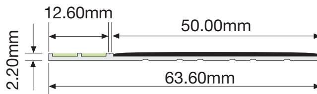
**The E14-075 Step Edge Contrast is designed to ensure visibility of steps in escape routes for compliance with International Fire Code (IFC), and any performance based building codes. The Step Edge Contrast will be effective in all light conditions including during failure of the main lighting.**
