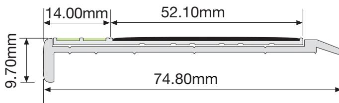
**The F14-175 Step Nosing is designed to ensure visibility of steps in escape routes for compliance with International Fire Code (IFC), and any performance based building codes. The Step Nosing will be effective in all light conditions including during failure of the main lighting.**
