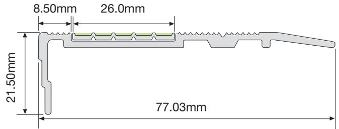
The F2-003 Step Nosing is designed to ensure visibility of steps in escape routes for compliance with NFPA 101 Life Safety Code (NFPA 101) and International Fire Code (IFC). The Step Nosing will be effective in all light conditions including during failure of the main lighting.
