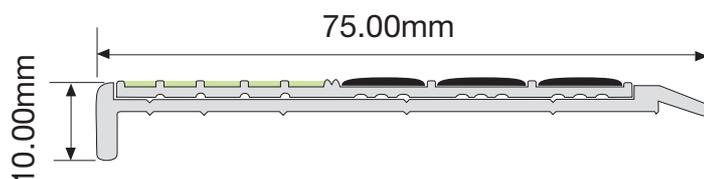
**The F14-173 Step Nosing is designed to ensure visibility of steps in escape routes for compliance with NFPA Life Safety Code (NFPA) and International Fire Code (IFC), and any performance based building codes. The Step Nosing will be effective in all light conditions including during failure of the main lighting.**
