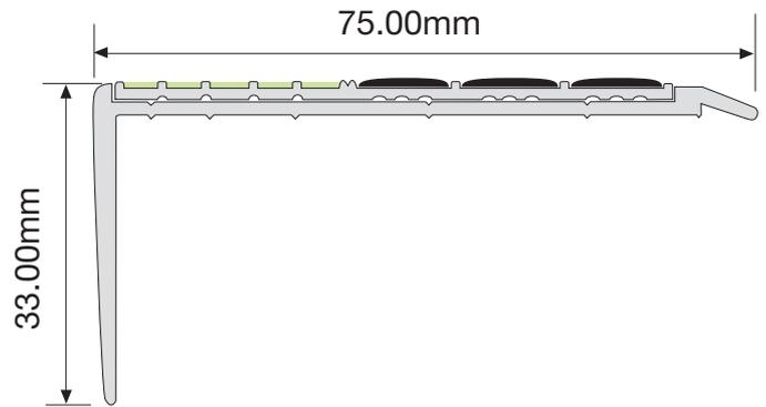
**The F15-173 Step Nosing is designed to ensure visibility of steps in escape routes for compliance with NFPA Life Safety Code (NFPA 101) and International Fire Code (IFC), and any performance based building codes. The Step Nosing will be effective in all light conditions including during failure of the main lighting.**
