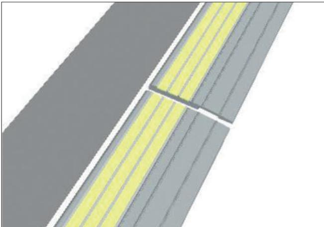
*Note: The Path Markers come in 1m lengths. A 3mm expansion/drainage gap must be left between lengths. Markers can be cut with a hand-saw or drop-saw to suit.*
