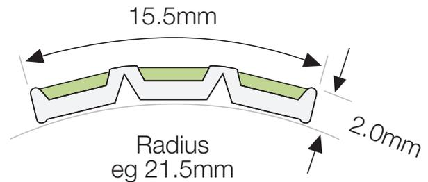
The H3-001 Handrail Marker is designed to ensure visibility of specified building features in escape routes for compliance with NFPA 101 Life Safety Code (NFPA 101) and International Fire Code (IFC), and any performance based building codes. The Handrail Marker will be effective in all light conditions including during failure of the main lighting.
