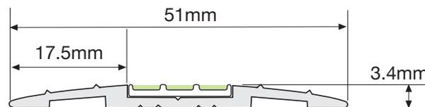
The T5-101 Path Marker is designed to ensure visibility of specified building features in escape routes for compliance with NFPA 101 Life Safety Code (NFPA 101) and International Fire Code (IFC), and any performance based building codes. The Path Marker will be effective in all light conditions including during failure of the main lighting.
