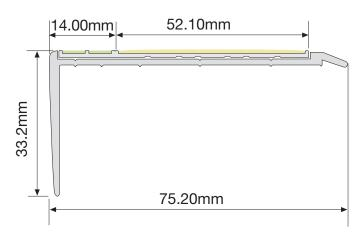
The F15-155 Step Nosing is designed to ensure visibility of steps in escape routes for compliance with International Fire Code (IFC), and any performance based building codes. The Step Nosing will be effective in all light conditions including during failure of the main lighting.
