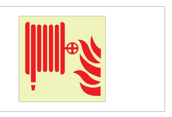
Ecoglo S5 Fire Hose Sign is designed to be used in and about buildings, structures and facilities to identify the location of fire hoses. The sign will be readily and clearly visible along normal paths of travel, including exits.
