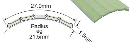
**H5-001-1000** Polyurethane adhesive fixing
