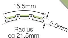
**H3-001-1000** Polyurethane adhesive fixing
